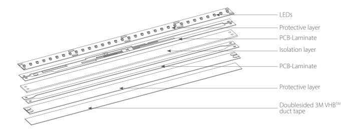
Supply method: The maximum length of the section fed in series is 5m.
