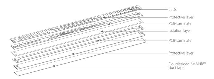
Supply method: The maximum length of the section fed in series is 5m. This product must be installed in an aluminum profile or other material with good heat dissipation. On request, possible sections: 30m or 50m
