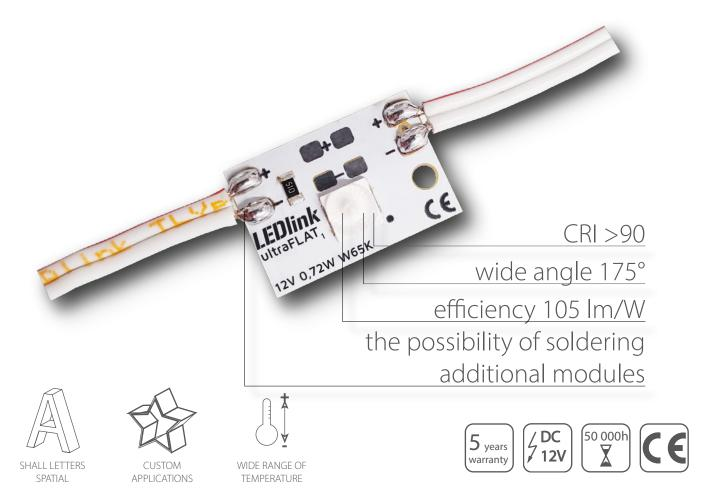
The ultraFLAT<sub>1</sub> is a compact module for indoor use. It is ideal for extremely flat lightboxes and profile letters. The module has a special 175° lens, which directs the light almost exclusively to the sides and thus guarantees a homogeneous illumination. The design of the module allows very flexibly and fast on the spot soldering more modules.
